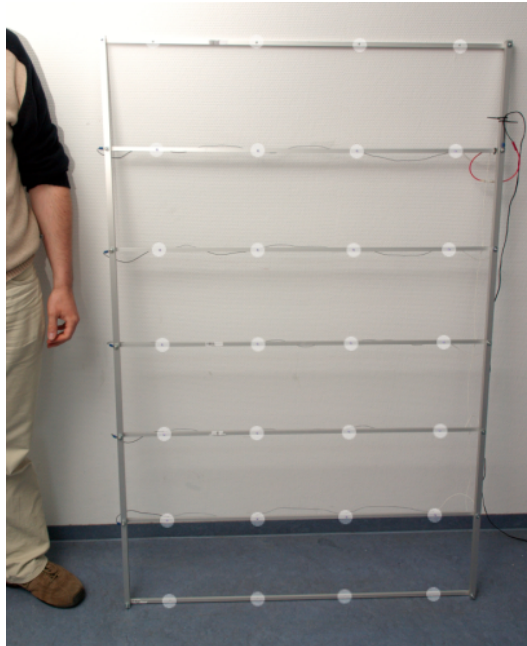
Figure 4.10: Overhead light source (LEDs highlighted)
