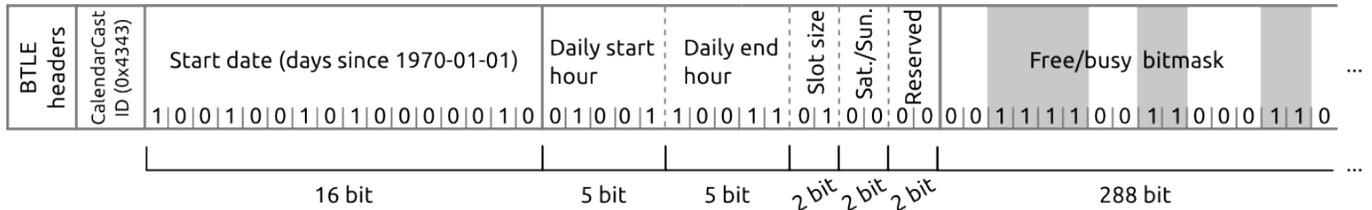
Figure 2. Bit-level description of CalendarCast message format (all numbers represented in network byte order, i.e. big endian format as suggested by [14]). This message is split and encapsulated in two BTLE broadcast frames.
