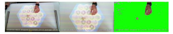
Figure 2. SurfaceStreams sends rectified and background-subtracted depth camera video via GStreamer (left: raw video with projected game board and physical tokens, center: rectified to projection area, right: background replaced by chroma-key).
