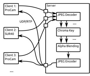
Figure 3. SurfaceStreams dataflow for example scenario.
