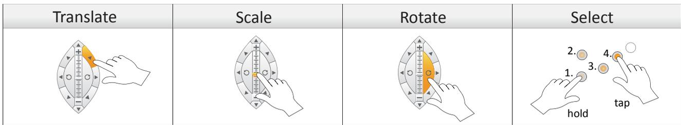
Figure 3: The control widget combines translation, rotation and zooming functionality in one shape.
