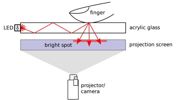
Figure 2. FTIR principle of operation
