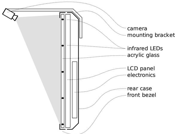
Figure 4. Schematic view (not to scale)
