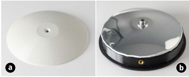
Figure 10: a) 3D-printed thermoforming mold. Printed at 0.08mm layer height. The central hole improves suction during vacuum forming and is used as a screw hole for fastening the mirror. [Printed on a common FDM printer (Prusa Mini) using a 0.25mm nozzle] b) The formed mirror is fixed to the mold, excess material is removed and the mold is screwed to an enclosure element. Permanently bonding mold and fixture guarantees dimensional accuracy and allows precise alignment.
