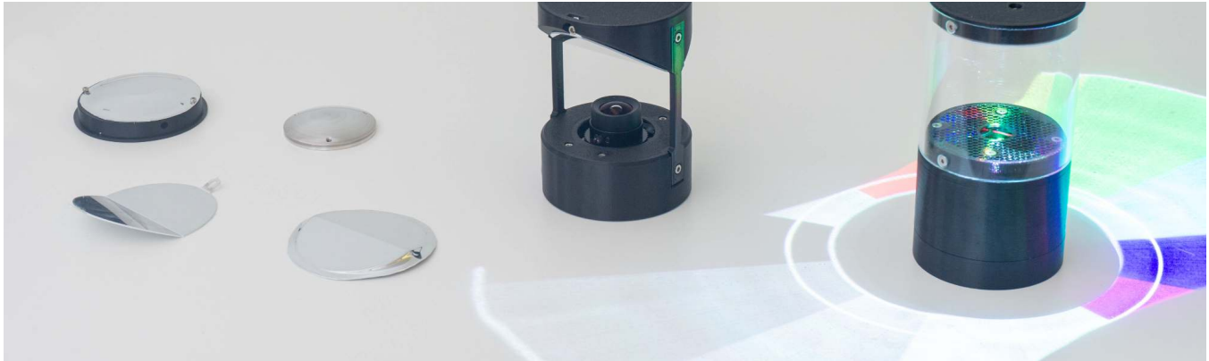
Figure 1: To decrease size or increase the field of view, mirrors are used to optimize the optical path geometry. This is often the case for small and mobile prototypes such as tangibles. Laminated polystyrene mirrors mounted on fixtures are suitable for usage with cameras and projectors alike.
