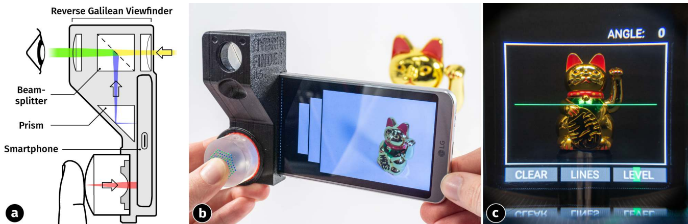
Figure 9: a) Cross section of the hybrid viewfinder. The beamsplitter overlays the light emitted by a section of the smartphone screen (blue) over the viewfinder image of the world (yellow), while the silicone attachment rests on the front camera (red). b) The finder can be slid over the top section of the smartphone. The silicone attachment provides rich tangible input to control settings and take a photo without visual confirmation as a touchscreen would require. c) View through the finder showing an overlay of the selection menu and a digital spirit level.
