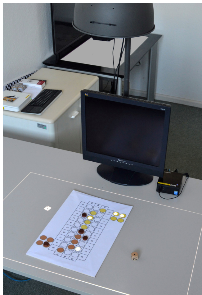
Figure 4: Projector/camera lamp (visible at top), with physical game board and projected token/dice markers.
