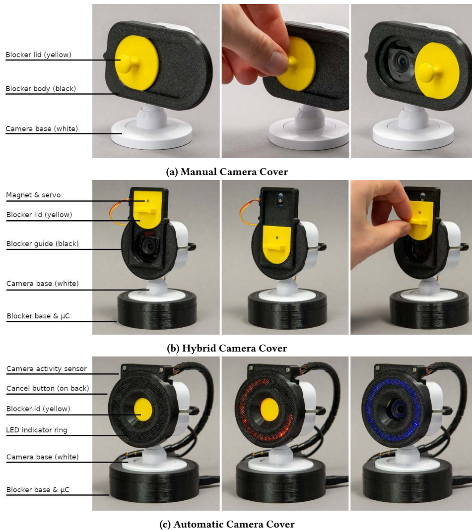
Figure 2: The three cover prototypes as add-ons to a Blink Mini smart home camera. The manual cover (a) requires to manually move the cap. The hybrid cover (b) lets the cap slide down automatically, but requires the user to manually lift it before next usage. The automatic cover (c) makes use of a motorized cap that opens and closes automatically but displays a countdown using the LED ring (red: counting down, blue: recording), allowing to abort manually through a button press before opening.
