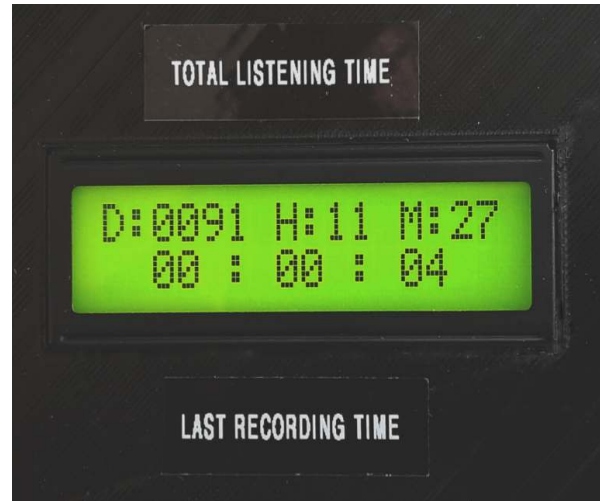
Figure 4: Closeup of VoxMox's LCD screen. The upper row displays time since activation and bottom row the duration of last interaction.
