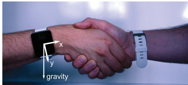
Figure 1: Exchanging contact data during handshake gesture. Alignment of gravity vector along y-axis of accelerometer is used to detect initiation of handshake.
