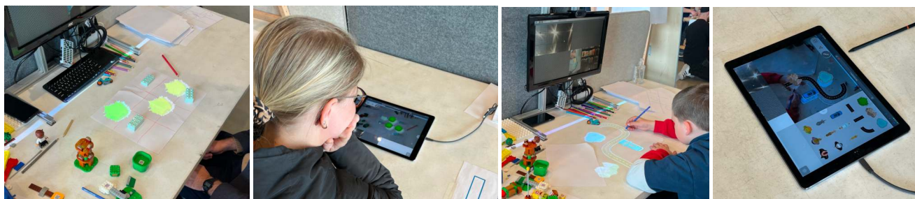
Figure 1: Collaborative play between spatially separate locations, using a projected tabletop (image 1/3) and an iPad (image 2/4). Left: the users have improvised a Tic-Tac-Toe game using physical Lego bricks and virtual stickers. Right: the iPad user is building a virtual road, which the child on the physical side uses as a drawing template.
